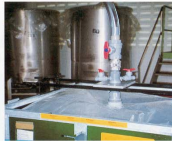
3. Filling from top into the liner.
